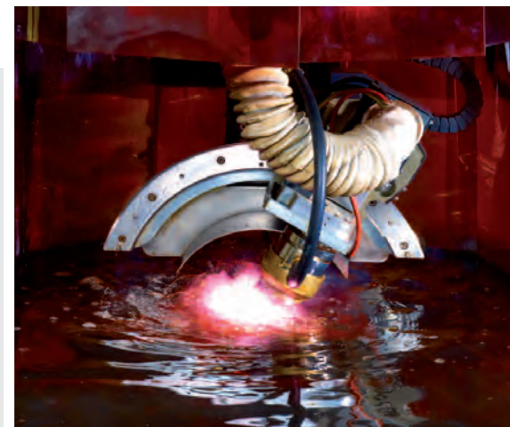
Plasma bevel cutting, under water with VBA Global PRO
